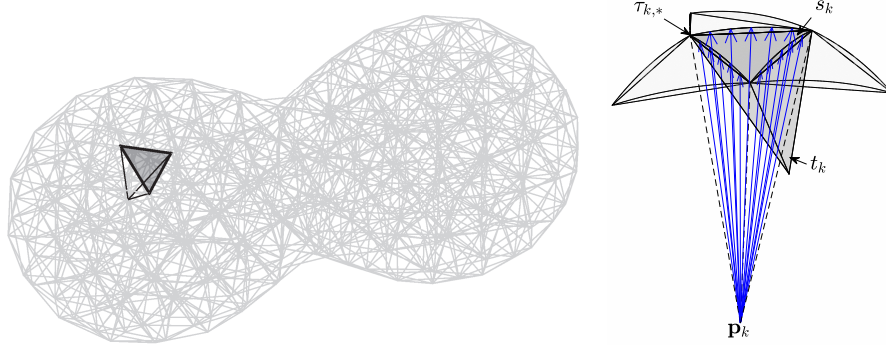
Figure 1: Left: A tessellation, T , of a point set, S_N , with a tetrahedron, t_k , at the boundary surface outlined in black. The triangular face \tau_{k,*} of t_k with three vertices on the bounding surface is shaded grey. Right: The projection procedure for the highlighted tetrahedron from the left frame. The arrows originating at \mathbf{p}_k indicate the projection of \tau_{k,*} 's edges to the surface. The dashed lines indicate the projection of \tau_{k,*} 's vertices from the projection point. When decomposing the volume \Omega the area of the triangle \tau_{k,*} , the areas between the arcs on the bounding surface and the edges of \tau_{k,*} , and the area of the curved triangle between these arcs make up the boundary of the sliver of volume, s_k , associated with t_k . The projection ensures that between adjacent slivers there are no gaps or overlaps, illustrated by the slivers of volume associated with three adjacent tetrahedra.
