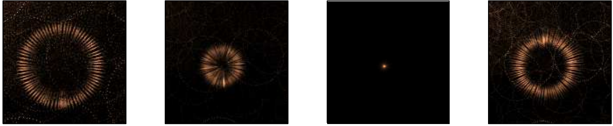
Figure 3. Reconstructions at 4 wavelengths to illustrate off-wavelength artifacts. The target is a pinhole in front of a white light source with a 20nm bandpass filter centered at 540nm. The wavelengths of reconstruction are (from left to right) 500,520,540, and 575 nm. The in-band reconstruction shows an image of the pinhole, but out-of band reconstructions create circles of radius f_3 (|\theta(\lambda_r) - \theta(\lambda_o)|) . The dimmer (off-center) circular artifacts are the result of uncorrected hot pixels in the camera.
