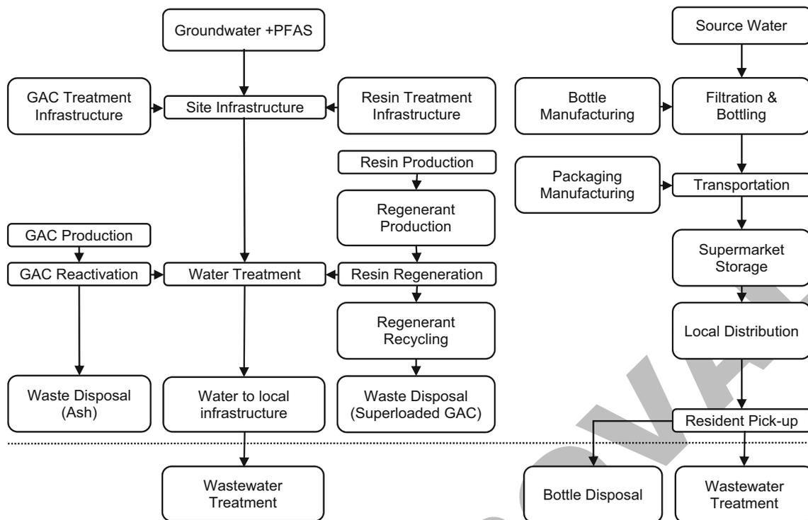
**Fig. 1** System diagram of stages included in life cycle assessment of water supply scenarios. Stages below the dashed line are not included in the analysis
