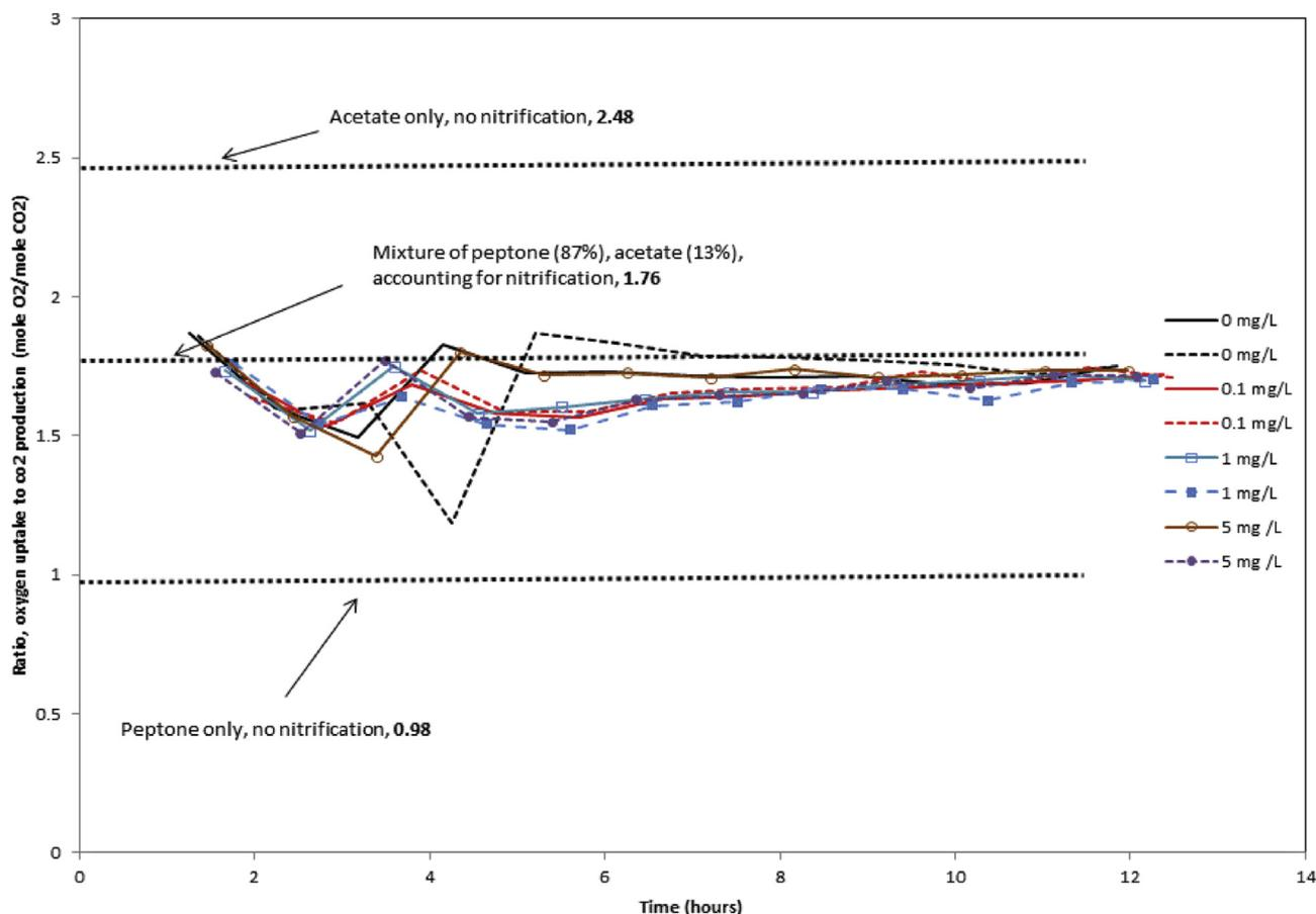
Fig. 2. The effect of malathion concentration on  $O_2$ -to- $CO_2$  molar ratio. Theoretically-derived ratios were determined for growth on acetate, peptone, or their mixture (COD weight basis). Data from duplicate experiments is shown for each malathion concentration.
