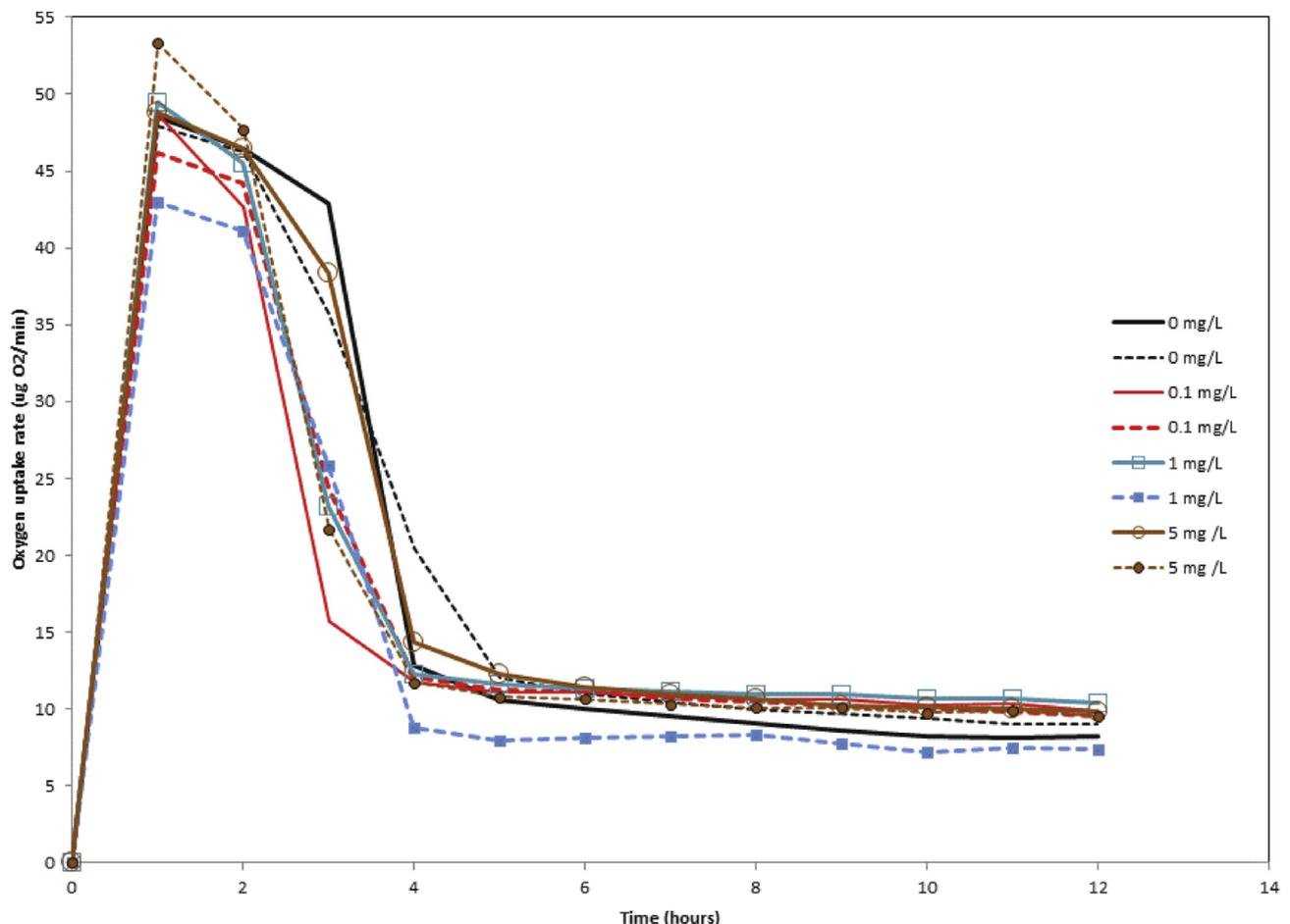
Fig. 1. The effect of malathion concentration on oxygen uptake rates during respirometry. Error for these measurements is  $\pm 2\%$ . Data from duplicate experiments is shown for each malathion concentration.
