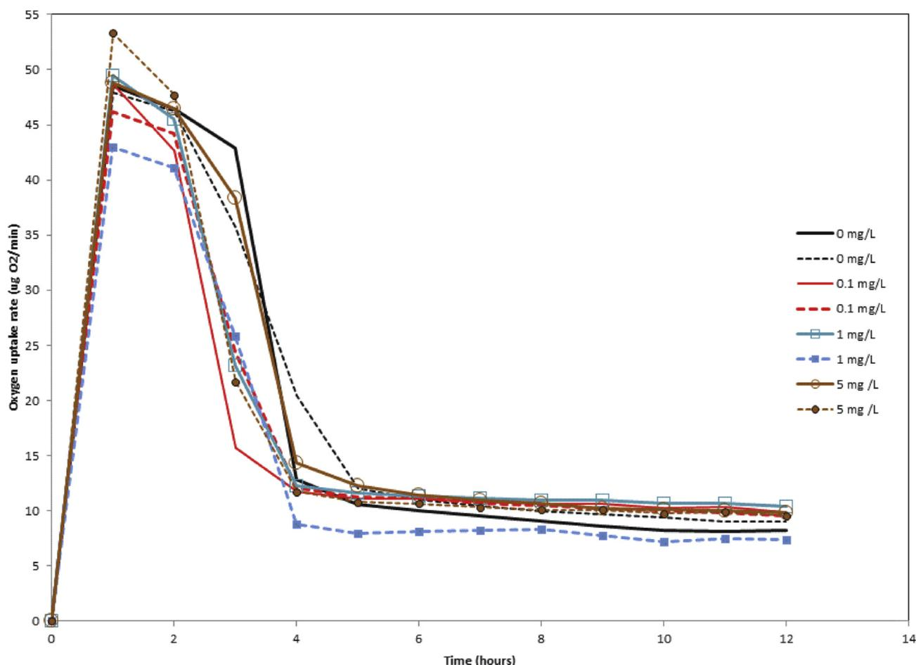
Fig. 1. The effect of malathion concentration on oxygen uptake rates during respirometry. Error for these measurements is  $\pm 2\%$ . Data from duplicate experiments is shown for each malathion concentration.
