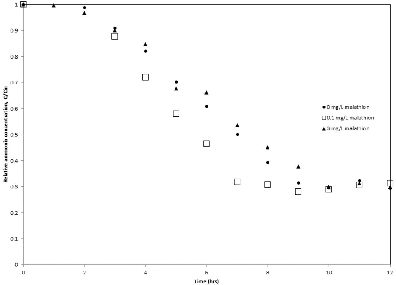
Fig. 4. Trial 1, The effect of malathion concentration on NH<sub>3</sub>-H removal in batch experiments.
