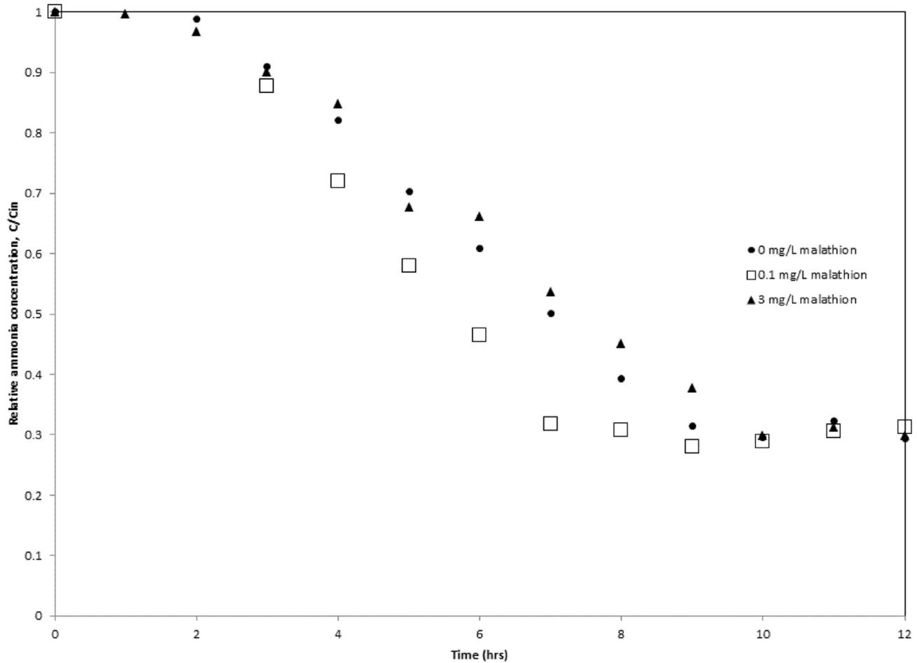
Fig. 4. Trial 1, The effect of malathion concentration on NH<sub>3</sub>-H removal in batch experiments.
