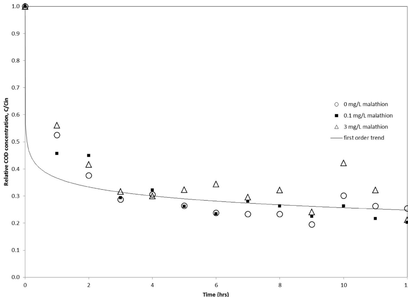
Fig. 3. Trial 1, The effect of malathion concentration on COD removal in batch experiments.
