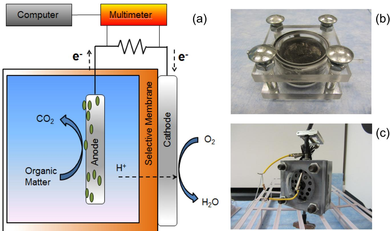
Fig. 1. (a) basic components of a single-chamber MFC; (b) view of anode chamber and carbon fiber anode; (c) configuration of electrode connections and external resistor.
