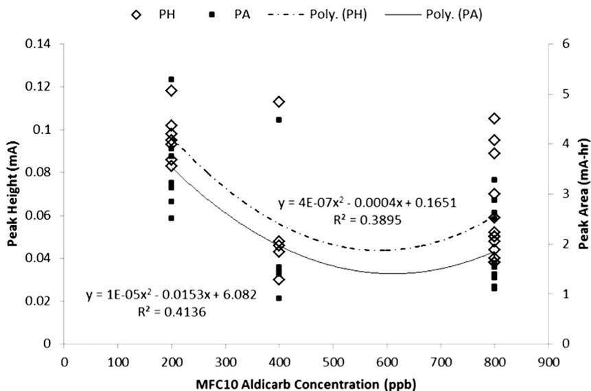
Fig. 3. PH and PA correlations with Aldicarb concentrations in MFC #10.
