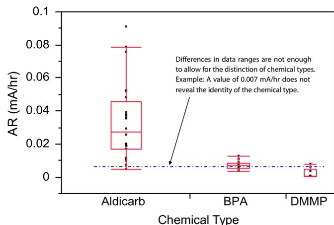
Fig. 5. The effect of chemical type on AR (mA/hr) in MFC #5.
