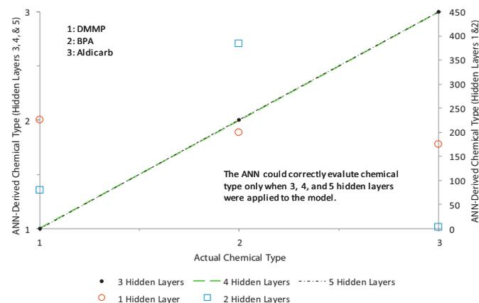
Fig. 6. ANN results for solvent effects testing using [PH, PA, AR, FrM] as the Input matrix for MFC #6.
