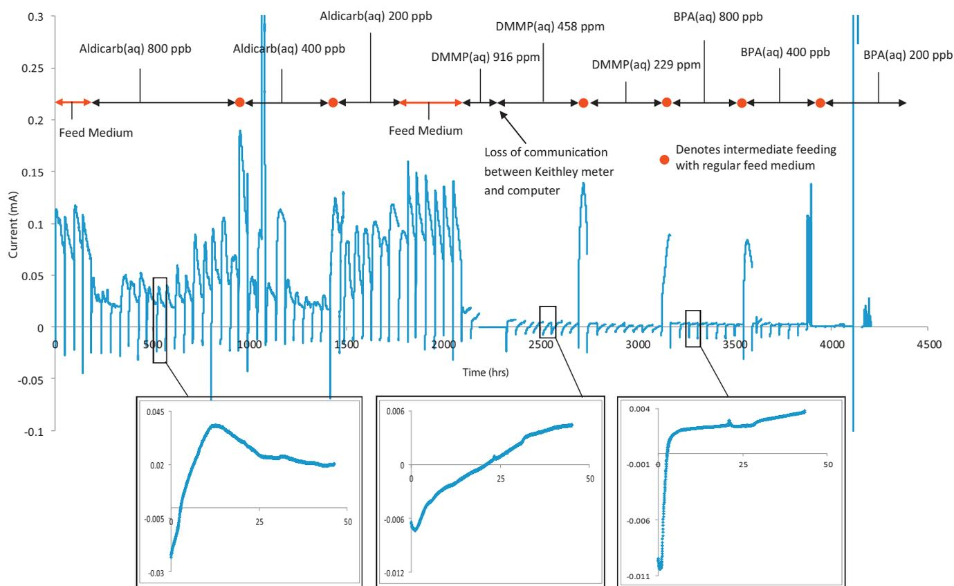
Fig. 2. MFC #10 operating history. (For interpretation of the references to color in this figure, the reader is referred to the web version of this article.)
