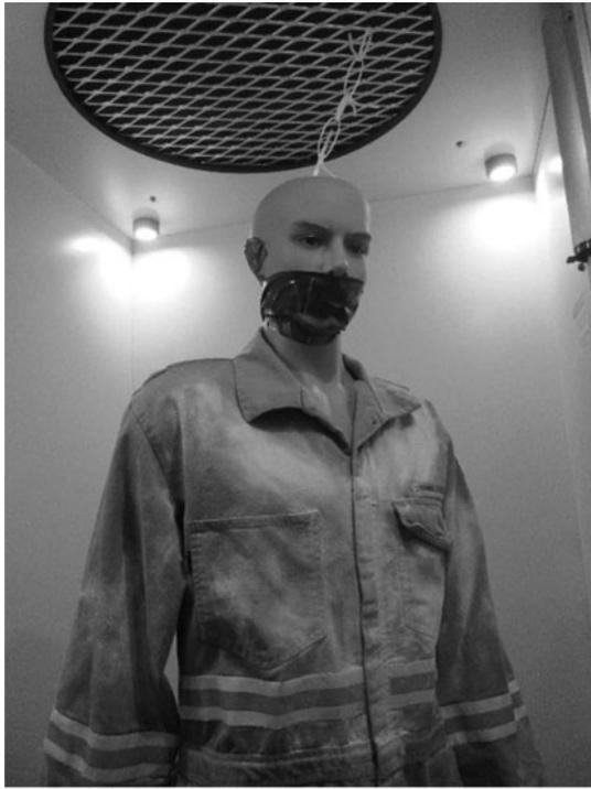
**Figure 2.** Air shower chamber with manikin showing the overhead air supply.
