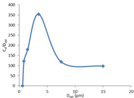
**Figure 3.** Example particle size distribution of sodium bicarbonate test dust.
