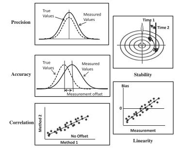
Figure 1 Basic measurement characteristics for quality assessment
