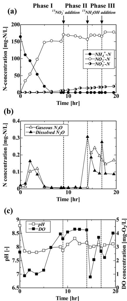
**Figure 1.** One-cycle profiles of ammonia oxidation and N<sub>2</sub>O production tests for nitrifying biomass acclimated in SBR: (a) nitrogen compounds; (b) gaseous and dissolved N<sub>2</sub>O; (c) pH and DO. The samples at 7, 14, and 17 h were taken right after the NO<sub>2</sub><sup>-</sup> and NH<sub>2</sub>OH spikes.
