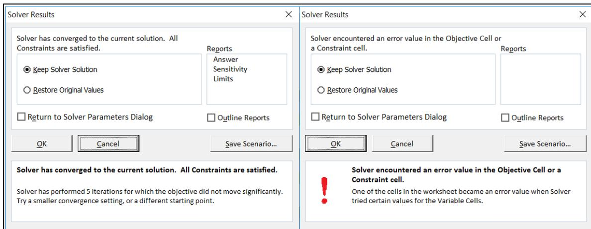
**Figure 5: Examples of good and bad Solver results**
