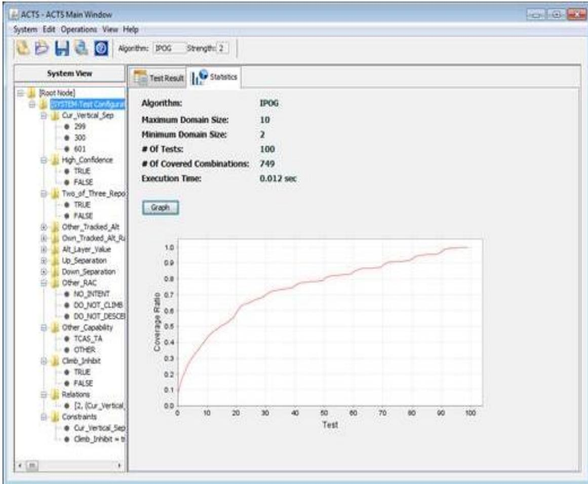
Figure 5: ACTS software shows coverage rate as test size increases
